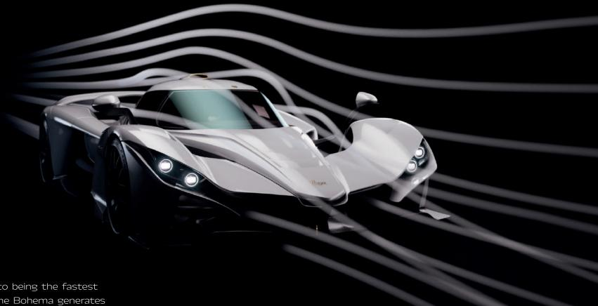
Aerodynamics are key to being the fastest through the corners. The Bohema generates 900 kg of downforce at 250 km/h.
