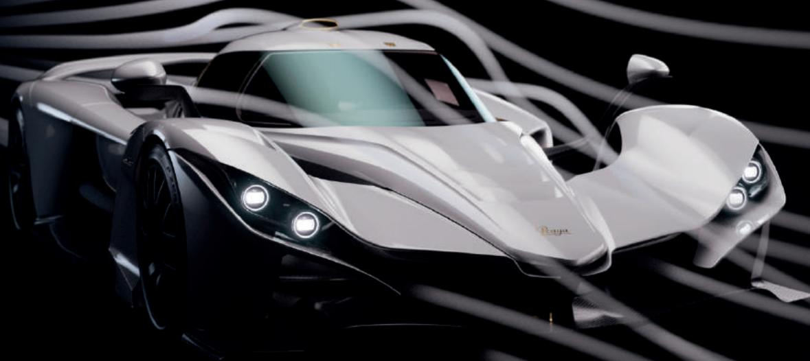
Aerodynamics are key to being the fastest through the corners. The Bohema generates 900 kg of downforce at 250 km/h.
